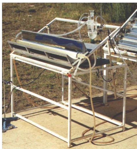
Fig. 1 The SOLFIN reactor and its schematic representation (see text for description).
